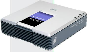
The SPA2102 is the latest dual FXS port analog VoIP adapter from Linksys. The SPA2102 features a built in router to separate your VoIP network from other devices or you can use the SPA2102 as your router to connect other devices to on your network.
